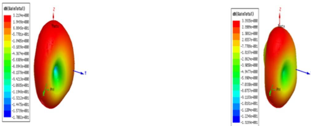
Fig-11. 3D Gain of UWB with WLAN notch
